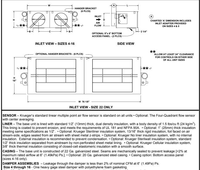
Size 22 – Two aluminum heavy gage opposed blades cross-linked with polyethylene foam gasketing.
